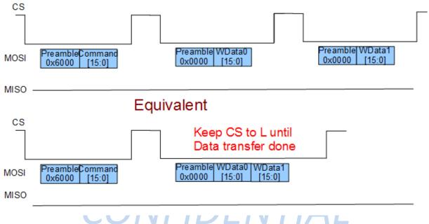
Both of above transfer type are available and equivalent in IT8951 SPI format.
